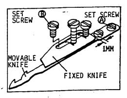
WHEN MOVABLE KNIFE MOVED TO ITS RIGHTEST DEAD POINT, THE HOOK BALDE OF MOVABLE KNIFE SHOULD BE RETREAT 1m.m. INSIDE FROM THE BLADE OF FIXED KNIFE.
